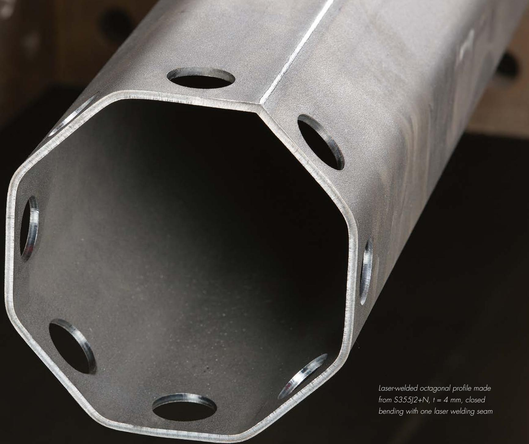
*Laser-welded octagonal profile made from S355J2+N,  $t = 4$  mm, closed bending with one laser welding seam*
