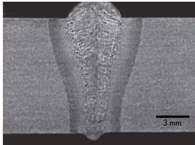
*Laser hybrid welding seam*
