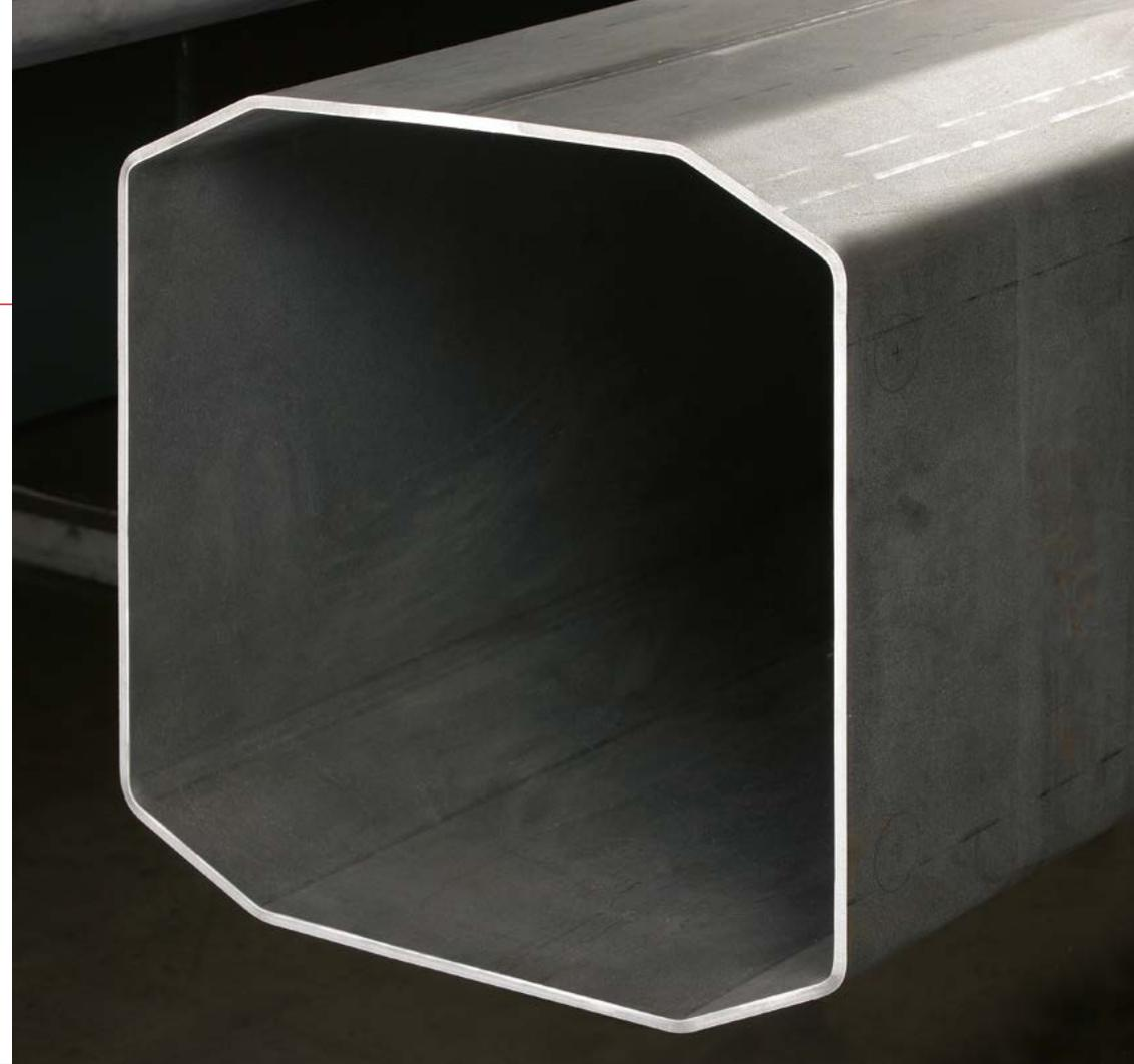
*Laser-welded octagonal profile made from S690QL,  $t = 8$  mm, closed bending with one laser welding seam*
