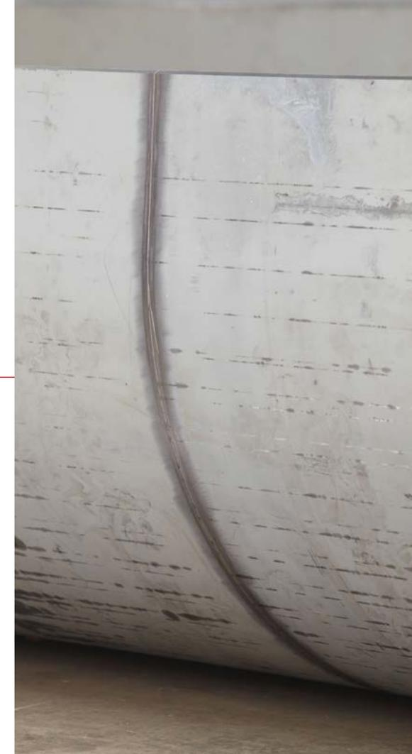
*S1100QL material with a plate thickness difference from 7 mm to 8.5 mm*
